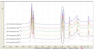
Figure 3. ATR-FTIR spectra of red fruit oil during high temperature treatment for acid value determination. The frequency region assigned with circle was used for partial least square (PLS) calibration model.
